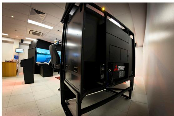
The VS-80PH70U feature Dynamic Brightness and Colour Balancing. Three built-in sensors continually monitor the Red, Green and Blue levels, then share this information with the adjacent cubes and adjust performance automatically for accurate balance over the entire display wall. This image uniformity helps to maintain the illusion of being on the bridge of a vessel.
